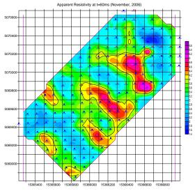
Figure 7. Apparent resistivity distribution at t=60 ms from second survey (Nov. 2006)
