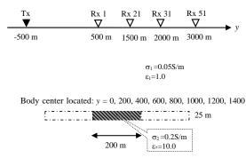
Figure 2 Model setup for water bearing reservoir
