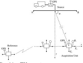
Figure 1 Array TEM survey setup
