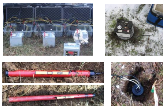
Figure 1. MT and gravity survey equipment: MT recording unit (upper left), AMT/MT coils (lower left), gravimeter (upper right), and electrical sensor (lower right).
