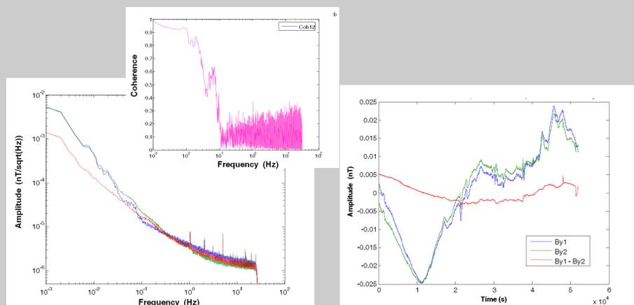
Fig. 9: Parallel sensor test with the digital fluxgate magnetometer at Hockley near Houston, left spectra, center coherence and on right time series with 14 hours recording.
