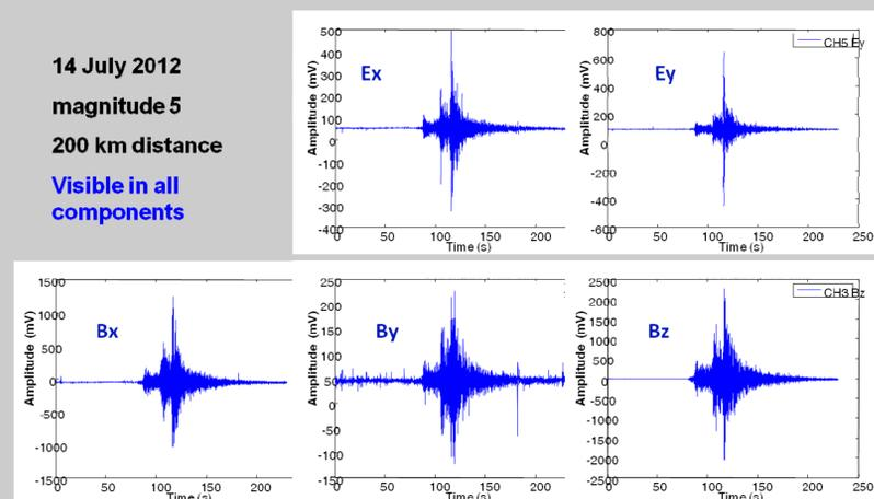
Fig. 10: Amplitude of electric and magnetic fields for all 5 components as function of time
