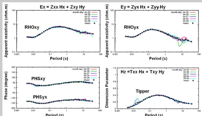
Fig. 2: MT response curves for 5 separated overnight recordings over a month at Hockley field test site near Houston.
