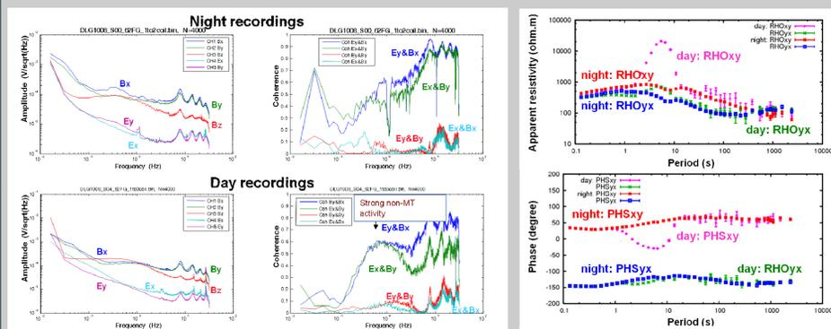
Fig. 11: Spectra (left), coherence (middle) and apparent resistivity & phase (right for night (top) and day (bottom) recording).
