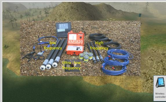
Fig. 1: Equipment of one MT station.
