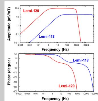
Fig. 3: system response for the Lemi-sensors
