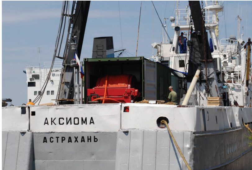
Fig. 3: CSEM transmitter winch on the back deck during the Caspian survey.
