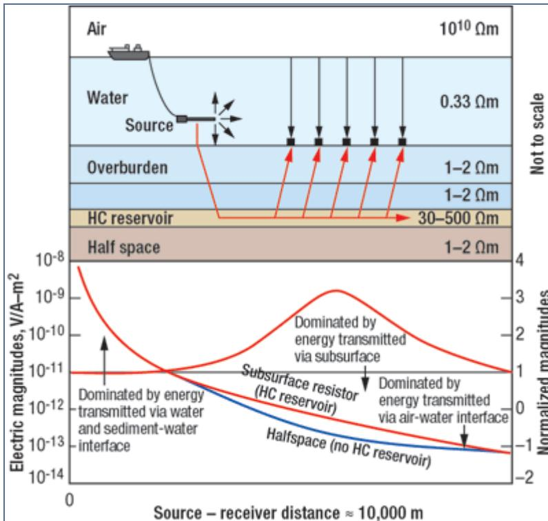
**Fig. 3.** Schematic of how CSEM works. Current propagates through the subsurface and to the receivers. Unwanted signal is minimized when optimum offset is used.<sup>5</sup>
