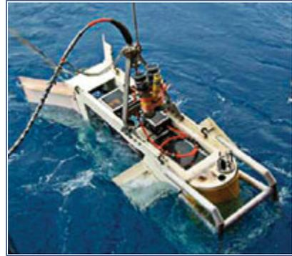
**Fig. 1.** Tow fish being deployed. It will power and monitor the electric dipole source streamer.<sup>5</sup>
