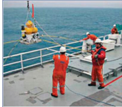
**Fig. 2.** Receivers being dropped to the seabed.<sup>5</sup>
