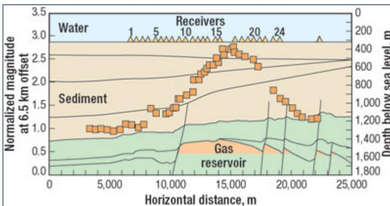
**Fig. 4.** Normalized MVO magnitudes, at 6 to 7 km, after median-filtering, across Troll West Gas Province, with receiver positions. Median normalized magnitudes (3.25 km from receivers at common midpoint) are plotted on a simple geological model, showing excellent correlation between SBL data and the reservoir.<sup>6</sup>
