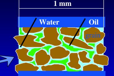
Oil is trapped by surface tension & structure.
