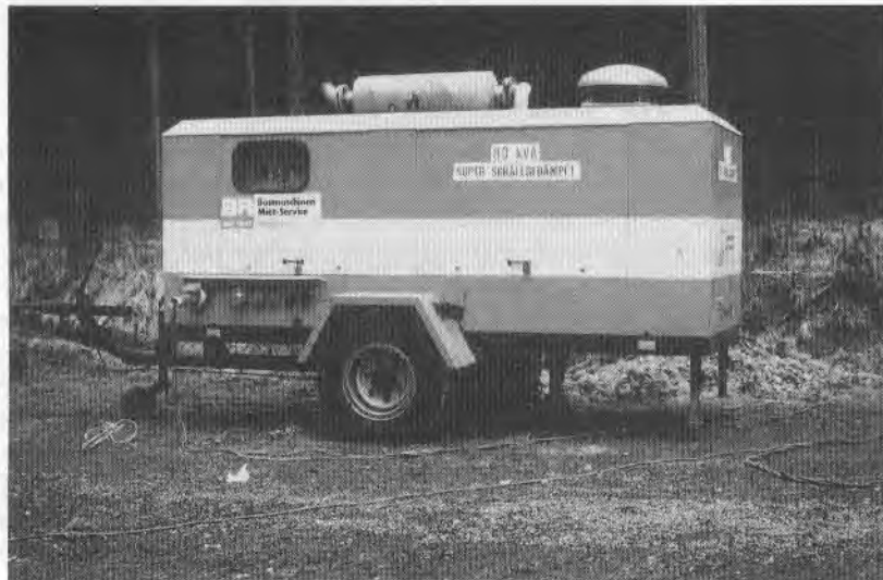
Fig. 5.9: Standard construction generator used for LOTEM test surveys in Germany.
