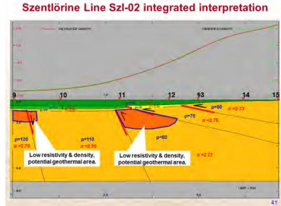
Figure 8: Sample gravity profile and integrated interpretation.
