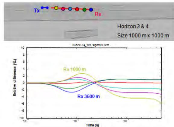
**Figure 3: Example for a 3D reservoir modeling Feasibility. The model combines three-dimensional seismic horizons and state-of-the-art 3D electromagnetic forward models. The surface transmitter is a dipole and the receiver offset is varied from 1,000 m to 3,500 m with respect to the model shown at the top.**
