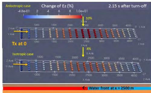
**Figure 3:** Time lapse Ez change above the waterfront at 2.15 s. after turn-off: anisotropic (top), & isotropic case when  $R_h = R_v$  (bottom).
