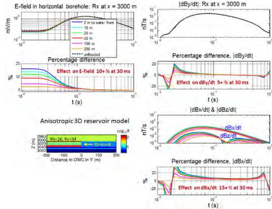
**Figure 8:** Borehole-to-surface: effect of approaching oil-water contact (OWC) to EM measurements on Bakken field.
