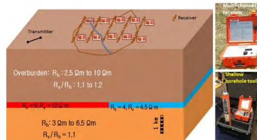
Figure 1: Flooded reservoir model and monitoring setup.
