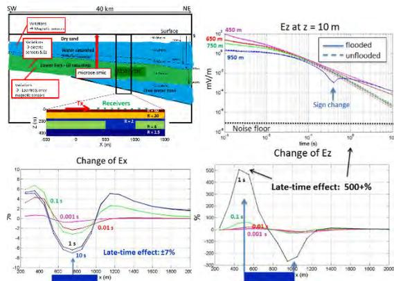
**Figure 2:** Heavy oil reservoir: steam-injection model (left top), Ex (left-bottom) and Ez (right) responses to the flooded area.
