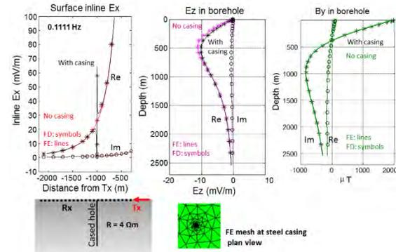
**Figure 9:** effect of steel casing on the EM field. Left: surface-to-surface; right: surface-to-borehole response; frequency: 1/9 Hz.
