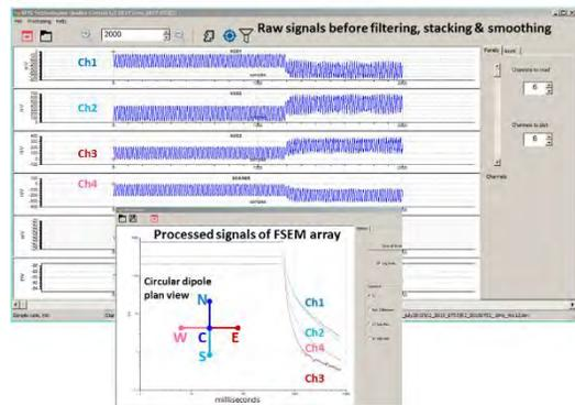
**Figure 10:** circular electric dipole, four-channel data processing: before (top) and after filtering, stacking and smoothing (bottom).
