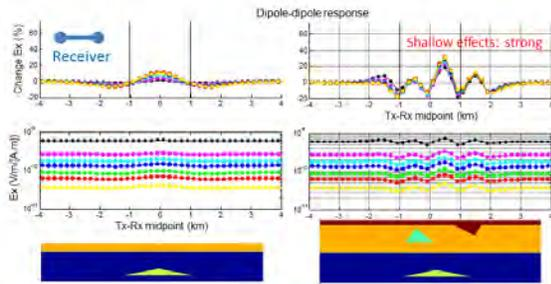
Figure 5: Papua New Guinea case: standard CSEM in the absence (left) and presence (right) of shallow structures. Tx-Rx offset: 1 km.
