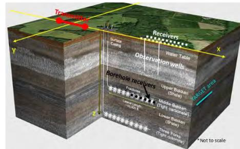
Figure 7: Bakken field 3D cross-section (courtesy of Miscoseismic Inc.) and monitoring setup.
