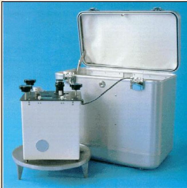
In **gravity** prospecting, we measure very small variations in the force of gravity from rocks within the earth. Different types of rocks have different densities, and the dense rocks have the greater gravitational attraction.
