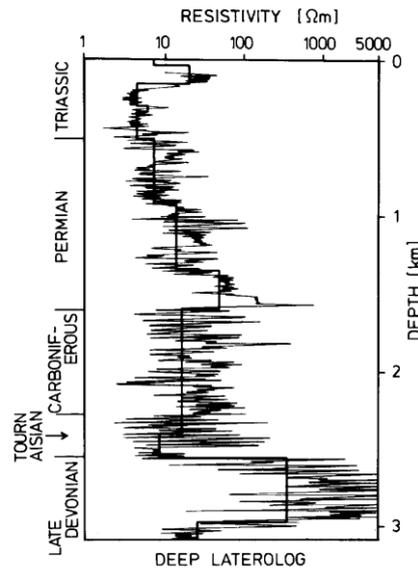
**Fig. 1. Resistivity log from the survey in Western Australia (Kora) and the equivalent resistivity model (heavy solid line). The layer boundaries were fixed using seismic interpretation (after Vozoff et al. [8])**
