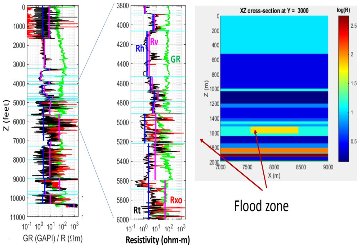
**Fig. 4. Generating a layered anisotropic model from a resistivity log. On the left superimposed on the logs is the blocky model. On the right is the cross section of the 3D model that includes also the reservoir zone (Flood zone).**
