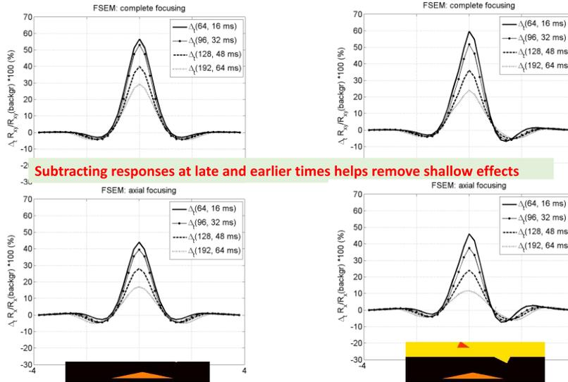
**Fig. 10. 3D model response along the profile above the model in Fig. 6 without (on the left) and with the near-surface structures (on the right). The unwanted shallow effects have been subtracted**
