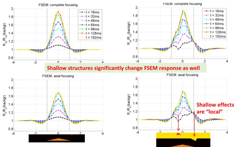
**Fig. 9. 3D model response along the profile above the model in Fig. 6. without (on the left) and with the near surface structures (on the right). The FSEM setup was used**
