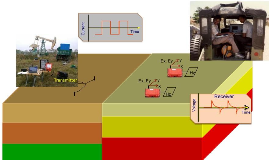
**Fig. 2. Typical survey setup for a CSEM system. Here, a time domain system is depicted with a grounded dipole transmitter and multi-component receiver. The respective current waveforms are shown for the square wave current injection and the received voltages (magnetic field exemplary). Also shown are picture of the equipment in the field**
