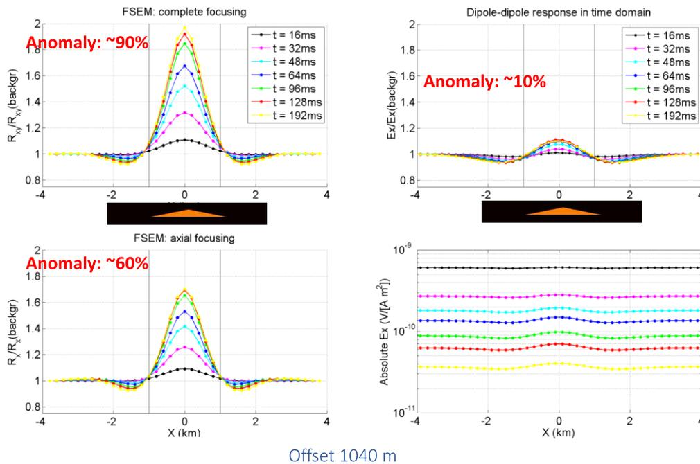
Fig. 7. 3D model response along the profile above the model in Fig. 6. for FSEM 'complete' and 'axial' focusing and standard Lotem inline electric fields
