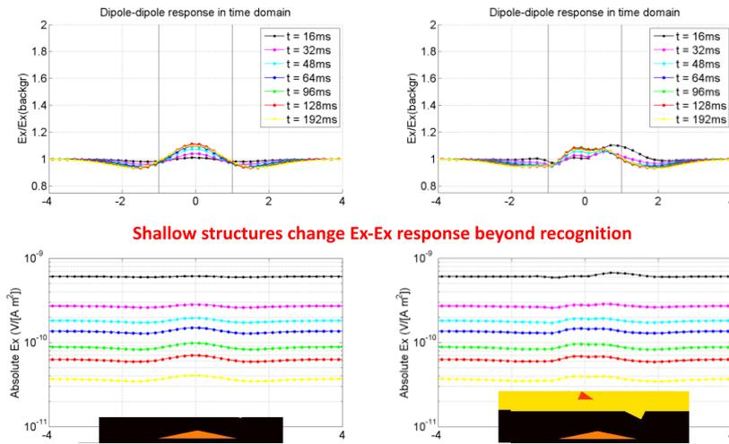
**Fig. 8. 3D model response along the profile above the model in Fig. 6. without (on the left) and with near-surface structures (on the right). The Lotem setup was used**
