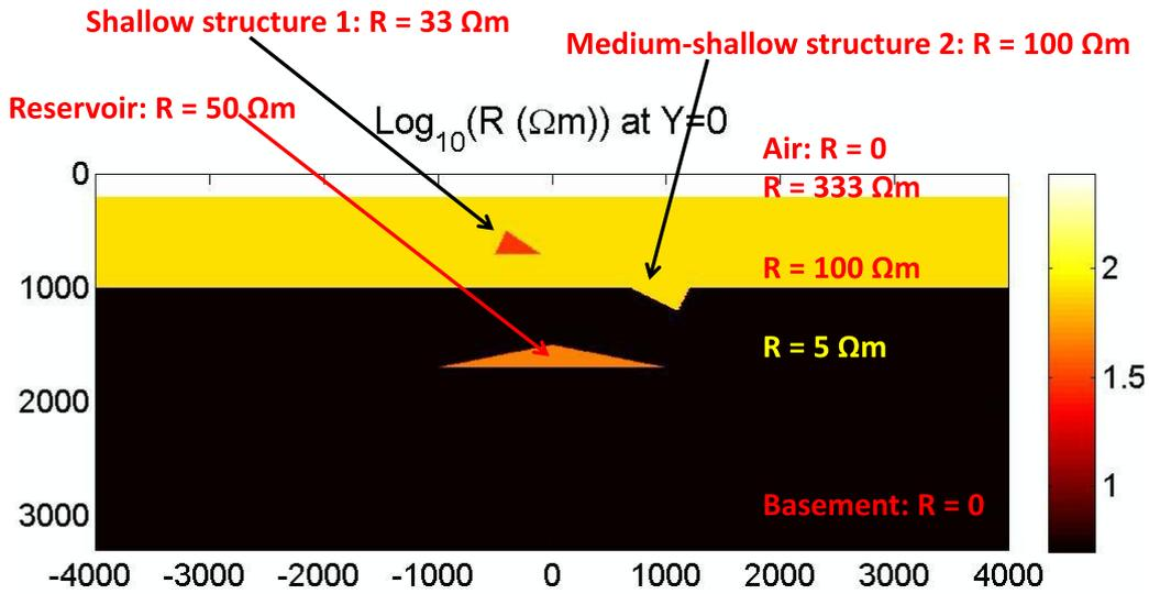
Fig. 6. 3D model setup of the carbonate model with near surface inhomogeneities. The resistivity values represent typical SE Asia carbonate fields
