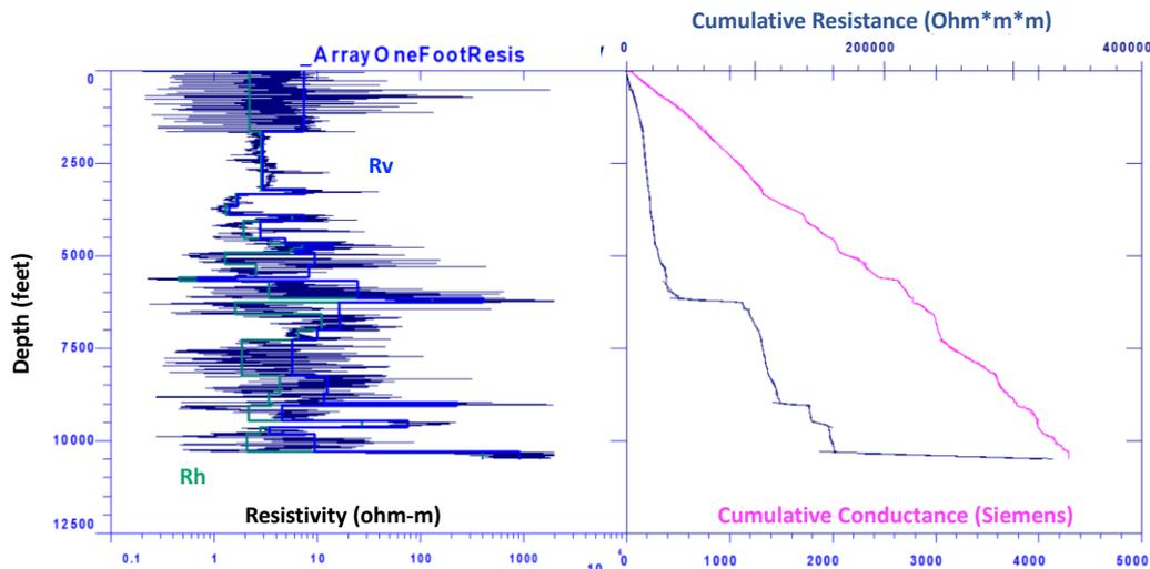
**Fig. 3. Example of analyzing the resistivity log and generating an anisotropic model. On the left: the model derived from the equivalent model resulted from fitting the cumulative curves on the right layer-wise**
