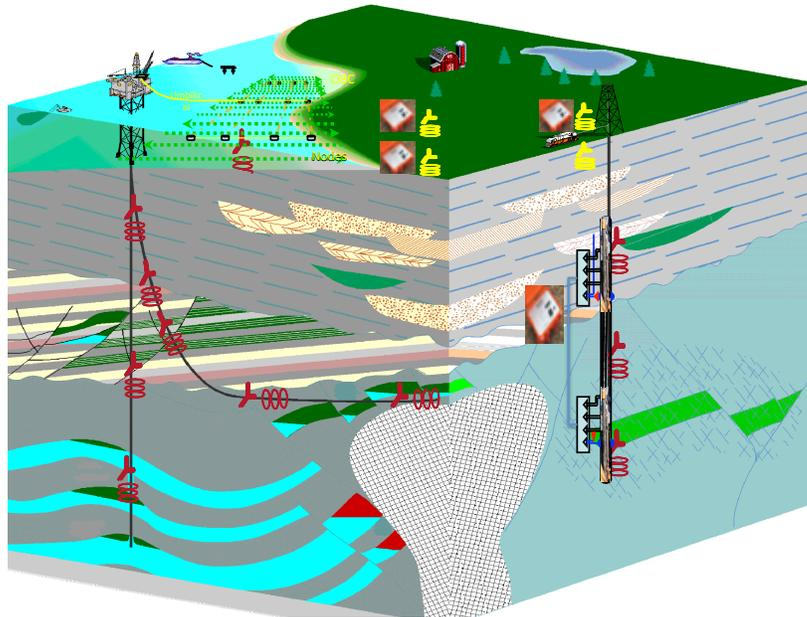
Figure 3: Artists rendition of Full Field Electromagnetics components. Sensors placed inside the borehole as well as on the surface (onshore and offshore) are shown.
