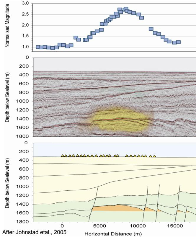
Figure 7: Example of a marine CSEM interpretation for the Troll field, Norway (after Johnstad et al., 2005). The top shows a magnitude versus offset curve, which exhibits an anomaly directly over the reservoir.
