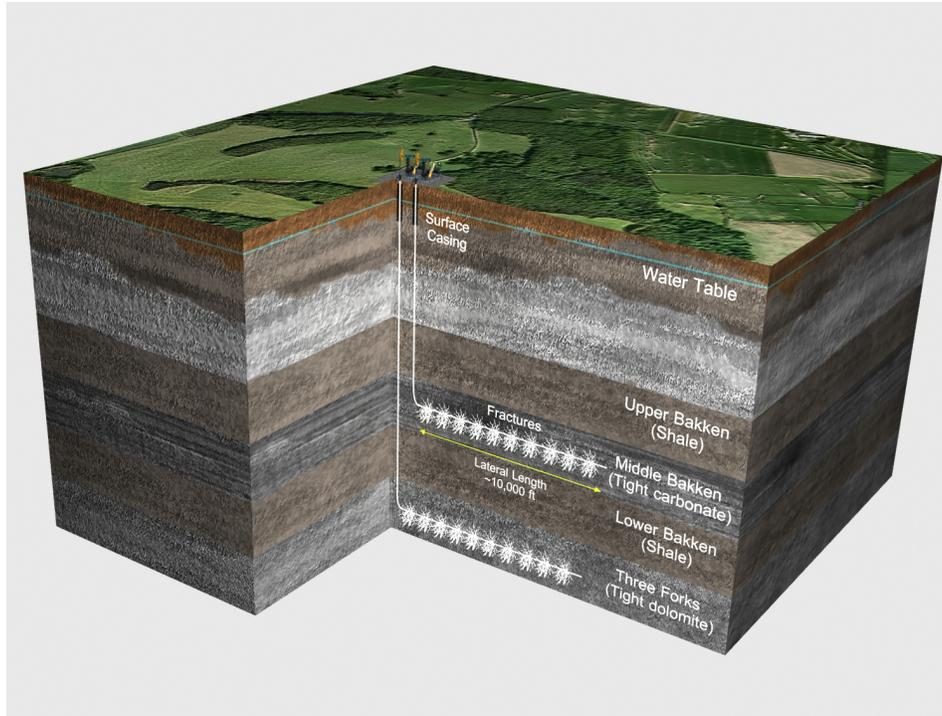
Figure 9: Sketch of a horizontal well in the Bakken formation used for the exploration and production in shale oil (After Statoil). The 3 Bakken formations are shown and the horizontal wells used for the development of the reservoir.
