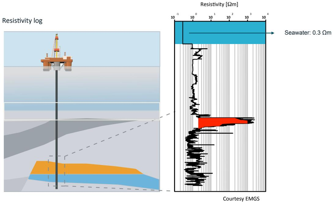
Figure 2: Sketch of a reservoir in a marine environment and an induction log. The induction log shows high resistivity in the reservoir zone indication high hydrocarbon saturations (courtesy EMGS).
