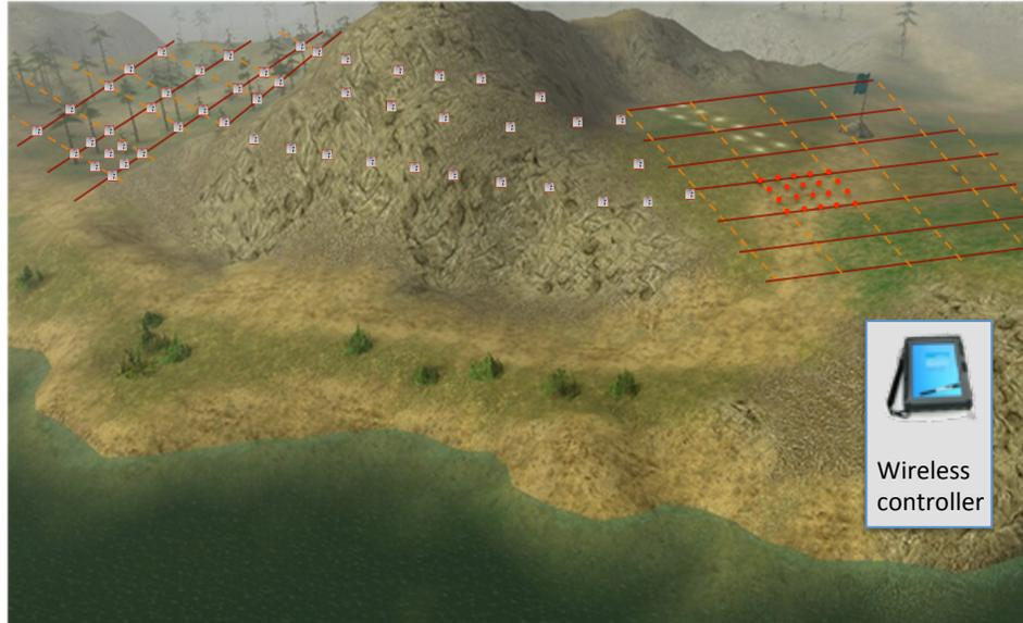
Figure 4: Seismic-style layout example of an electromagnetic survey using wireless nodes in a regular grid layout and also in irregular lines.
