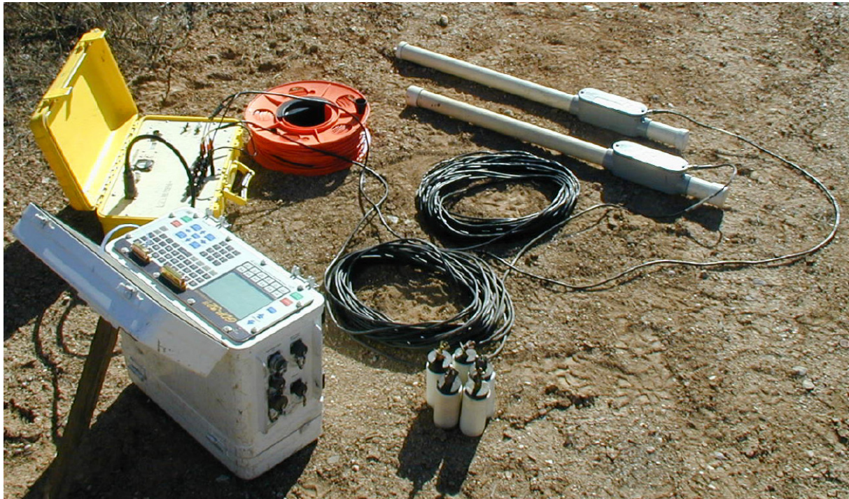
Figure 4. Photograph of equipment used for acquisition of MT data; a GDP-32 receiver unit (white case), SC-8 signal conditioner unit (yellow case), magnetic induction coils, porous pots, and signal wires.
