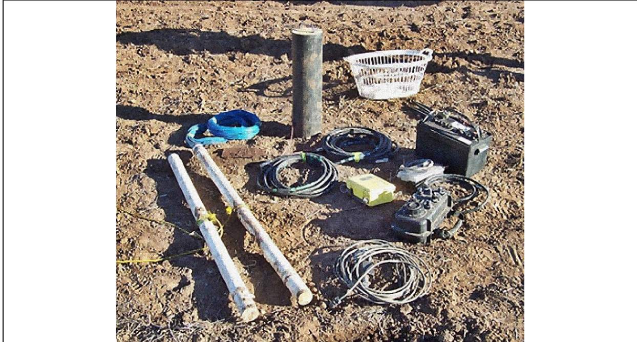
Figure 1. Typical equipment required for ground MT acquisition. Equipment includes horizontal magnetic field coils (long white cylinders), vertical field coil (short black cylinder), electrode connections, coil connectors, data logger, and battery power supply.
