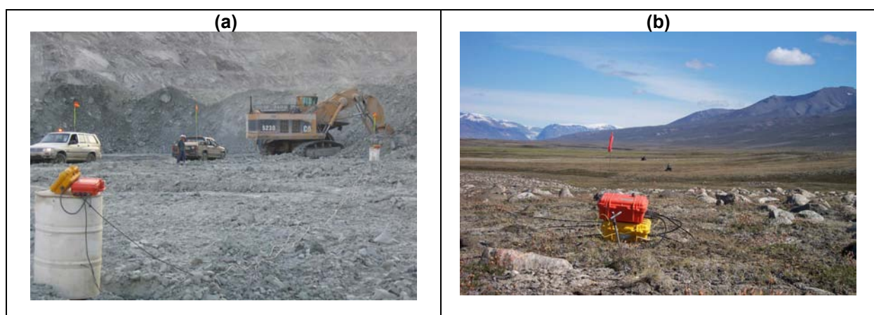
Figure 1. Photographs of (a) a Titan 24 array reading being taken in an operating pit in South Africa, and (b) a Titan 24 receiver and battery linked into an array for a survey in Greenland.
